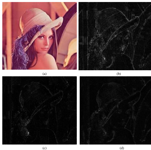
Figure 10 (a) Lena at 0.5 bpp and PSNR of 33.68 dB, (b) error image of the R component, (c) error image of the G component and (d) error image of the B component.
